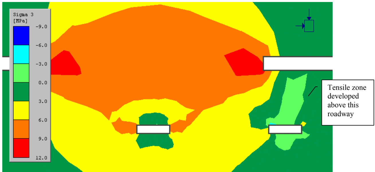
FIG. 7 - Development of tensile conditions above a roadway located adjacent to the goaf edge
